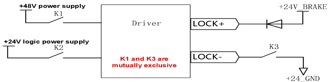
Figure 2-5 Recommended circuit wiring diagram for forced release brake
